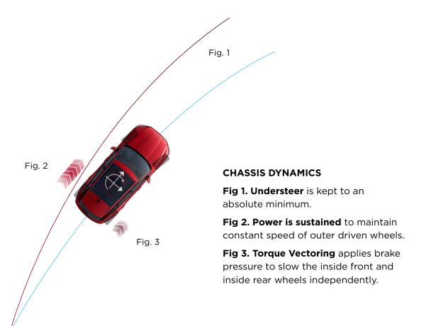
When straight roads become snaking roads, F-PACE's Torque Vectoring by Braking makes all the difference. It provides controlled independent braking on the inside front and rear wheels to maximise capability through even the tightest corners. Together with Dynamic Stability Control, it corrects understeer, giving the vehicle its sports car-like agility and providing you with extra confidence when driving.
